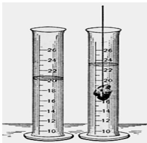
**Figure 1: The Law of Buoyancy: The buoyant force is equal to the weight of the displaced fluid<sup>(8)</sup>.**
